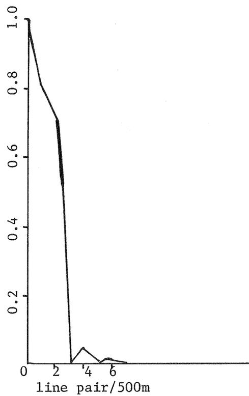
Fig.3. Example of calculation of MTF for MESSR
