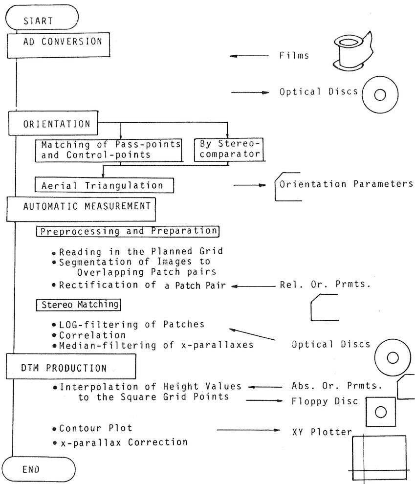
Fig.3 Flow of the automatic measurement
