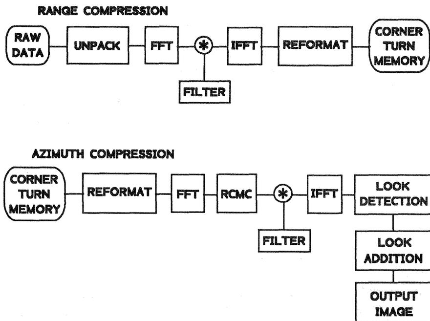
Figure 3-1 Block diagram of SAR algorithm.
