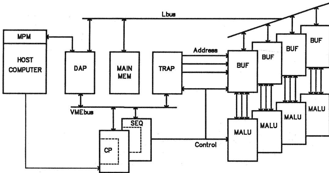
Figure 2-1 CESAR block diagram.
