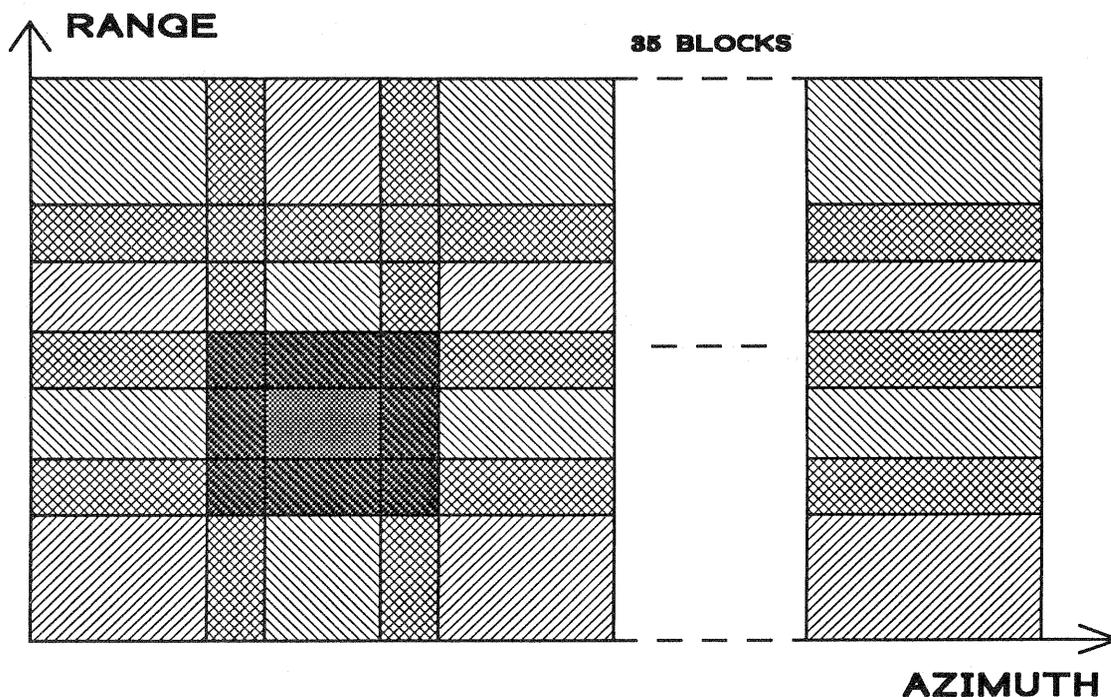
Figure 3-2 Division of scene into processing blocks.
