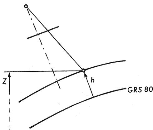
Fig.1 Projection of Imaging Rays on Reference Ellipsoid
