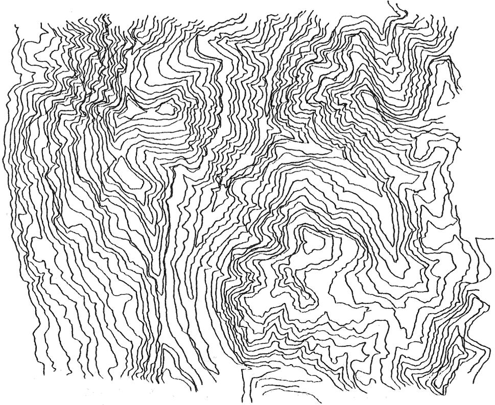
Fig. 6 : Test Area 'Vaduz' - Directly Plotted Contours
