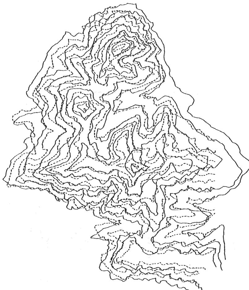
Fig. 8 : Comparison of Directly Plotted Contours ( solid ) and Map Contours ( dashed ) for Test Area 'Rottach-Egern' (approx. scale 1 : 61 000)
