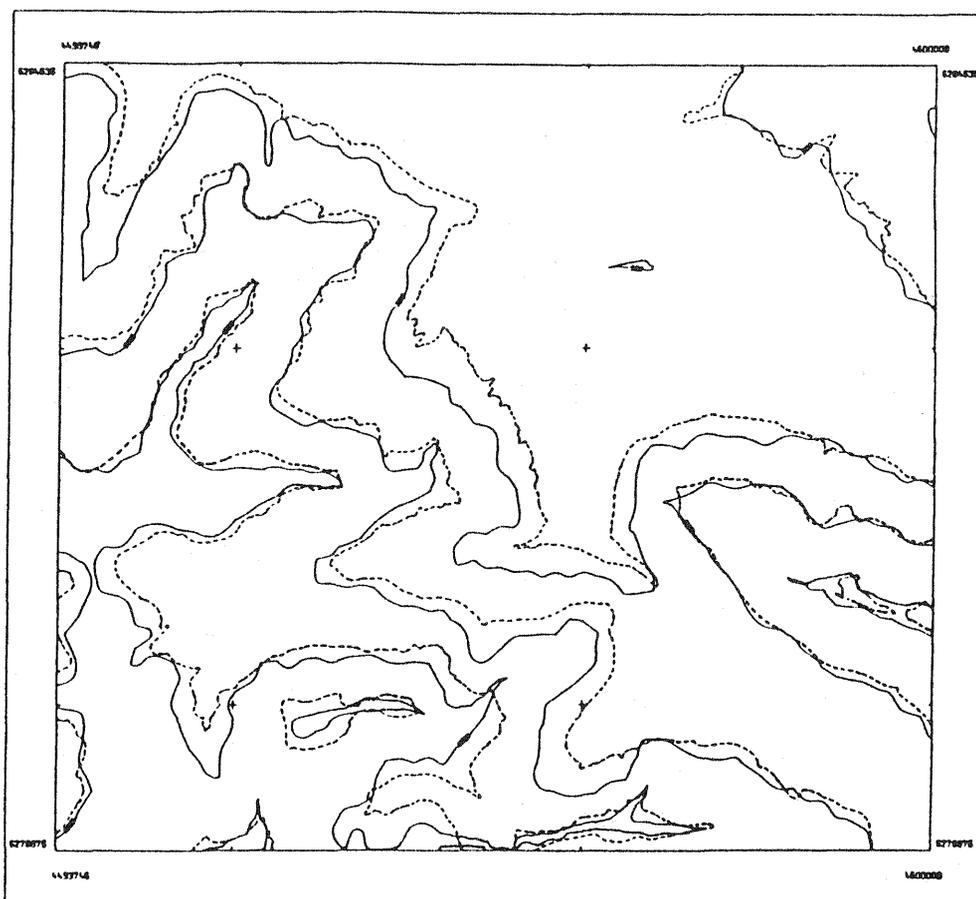
Fig. 2 : Comparison of Interpolated Contours ( solid ) and Map Contours ( dashed ) for Test Area 'Josefsthal' ( approx. scale 1 : 53 000 )
