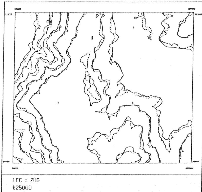
Fig. 3 : Comparison of Interpolated Contours ( solid ) and Map Contours ( dashed ) for Test Area 'Zug' ( approx. scale 1 : 61 000 )
