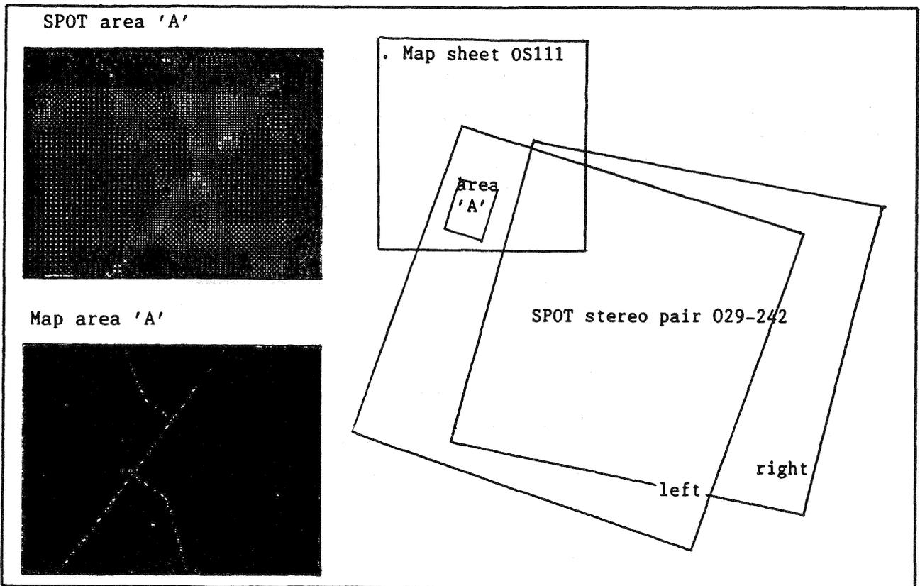
Figure 5: Initial registration of map and image by map transformation derived from orbital parameters
