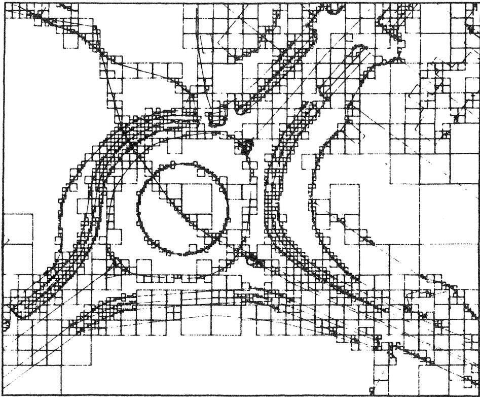
Figure 1: Visualisation of quadtree spatial index superimposed on map road features (UK map sheet 111)
