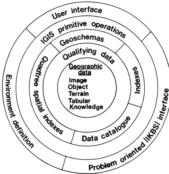
Figure 3: Schematic of integrated GIS system
