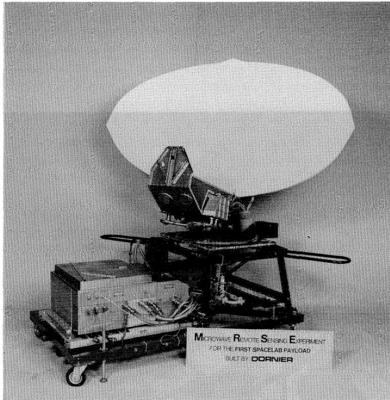
Fig. 2: Microwave Remote Sensing Experiment
