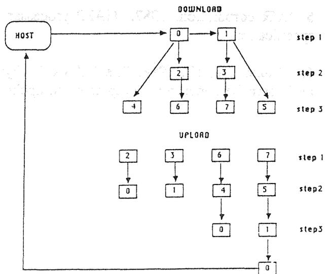
Figure 5. Data download/upload in an 8-node hypercube
