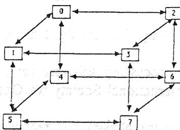
Figure 3. A 8-node hypercube connection
