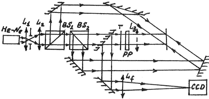
Fig. 4. Experimental setup for holographic filtering.
