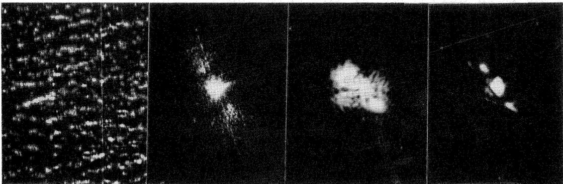
Fig. 8. The sea surface radioimage (a) and its spectra obtained with an immersion cell (b), without any filtering (c) and with IPH phase-noise filtering (d).
