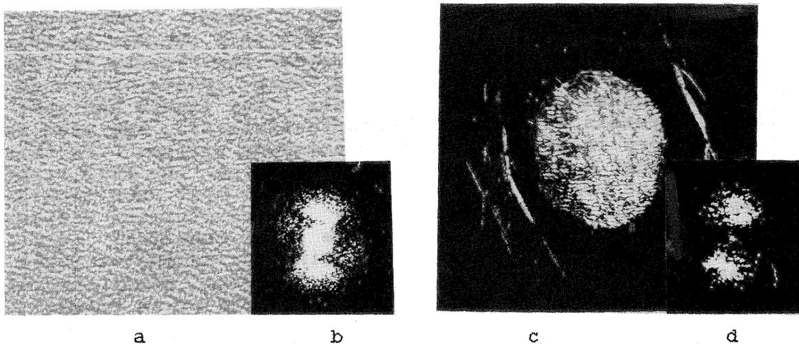
Fig. 2. The sea radioimage (a) recorded by the PRIZ (b) and its spectra (c, d).
