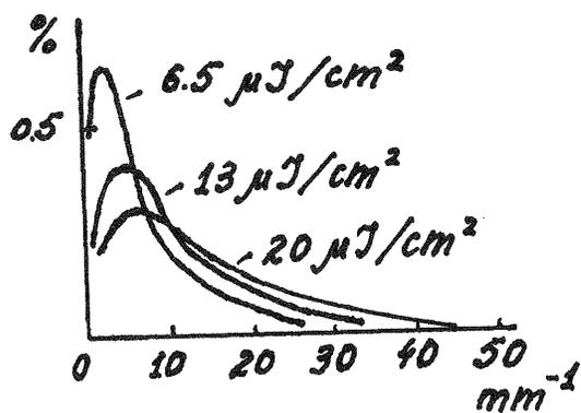
Fig. 3. PRIZ diffractive efficiency VS spatial frequency.
