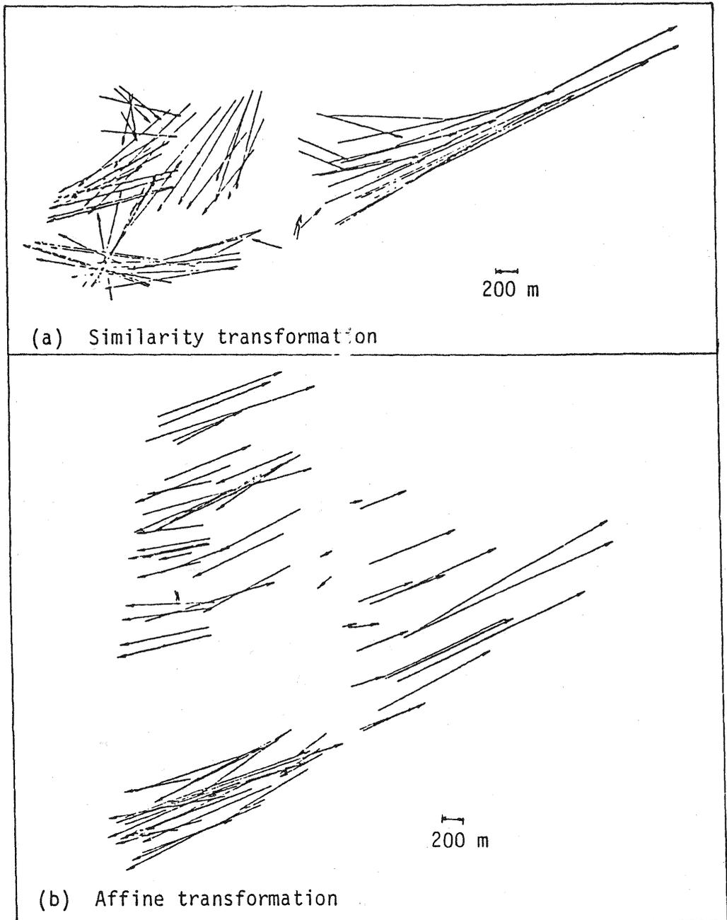
Fig. (4) Residual distortion vectors in the SAR formed block after similarity and affine transformations.
