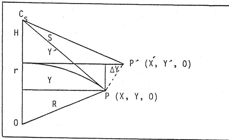
Fig. (2) Earth curvature -  $R$  = Earth radius;  $S$  = slant range to point 'P';  $H$  = satellite altitude
