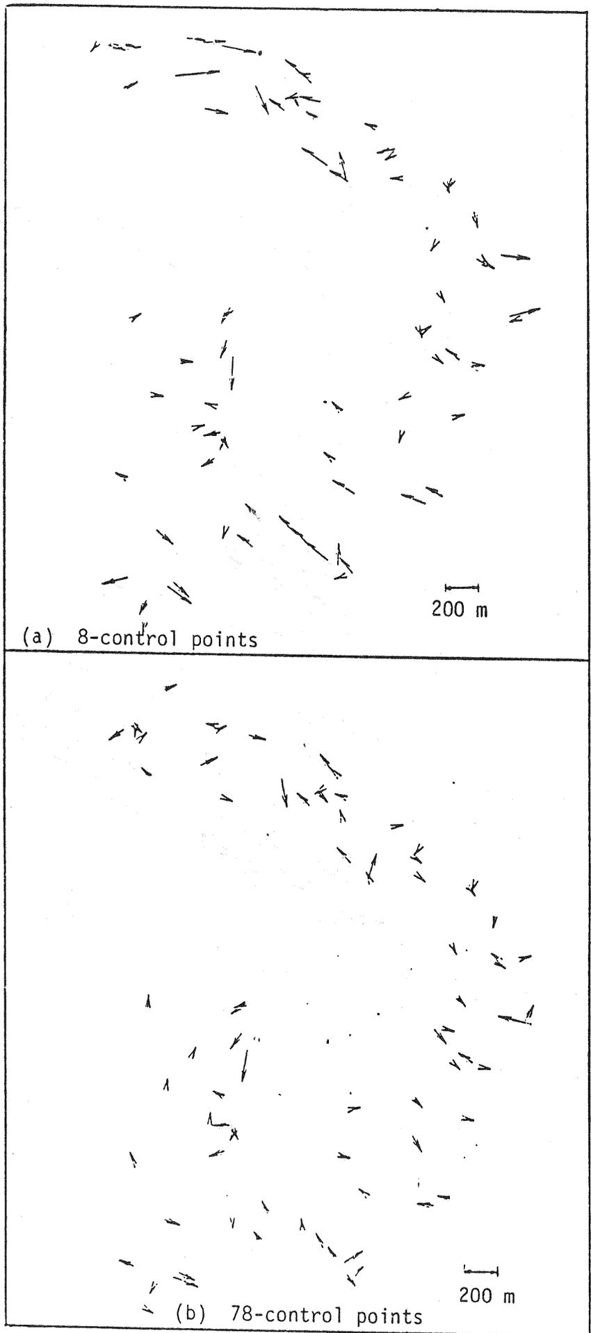
Fig. (5) Residual errors at the formed SAR block after; the proposed (theoretical) polynomials.
