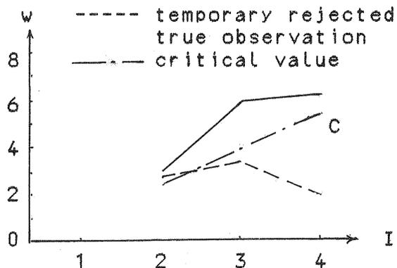
Figure 4 Changes in  $w$  of vertical control points with gross errors and temporary rejected true observations in four iterations
