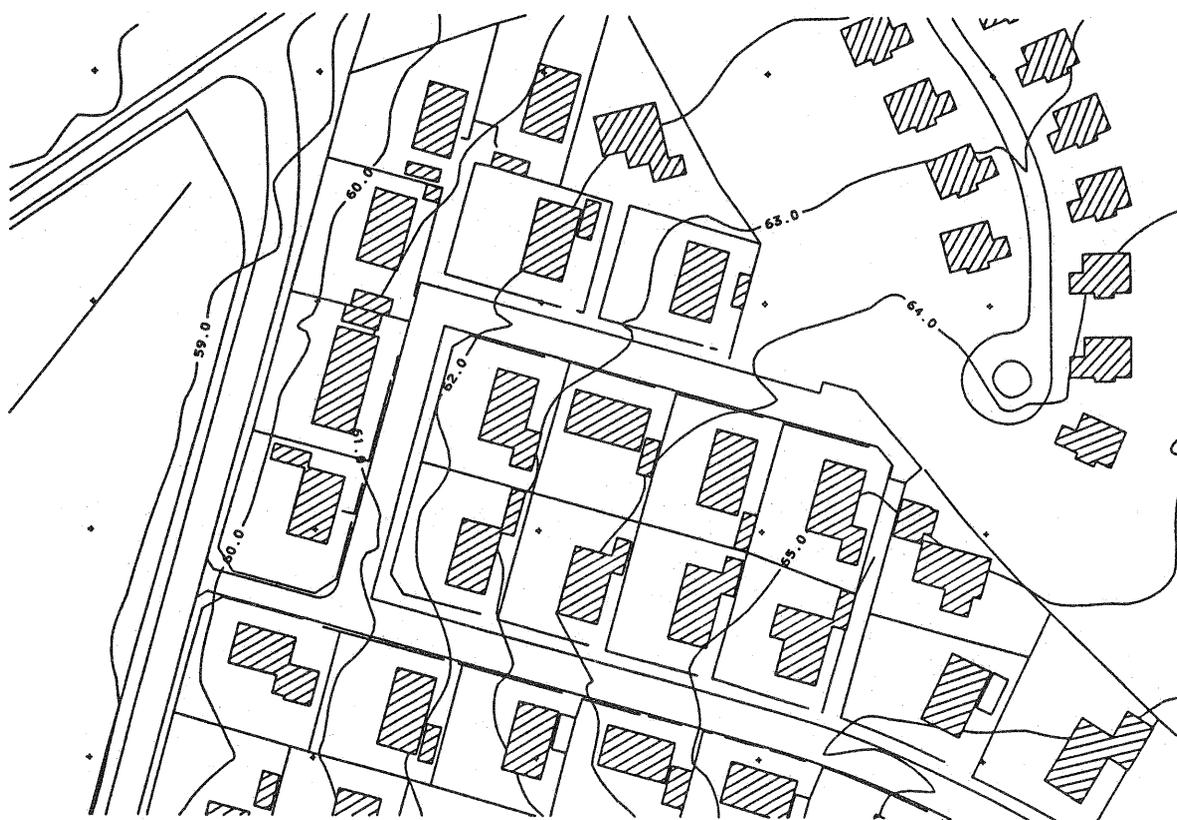
Fig. 4 Example of integration. The plot has been created in one step in program MAP. Houses, roads, etc. have been selected and plotted in the same session together with the contours.
