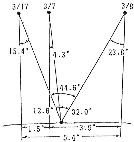
Fig. 1 Viewing angles of stereo triplet images
