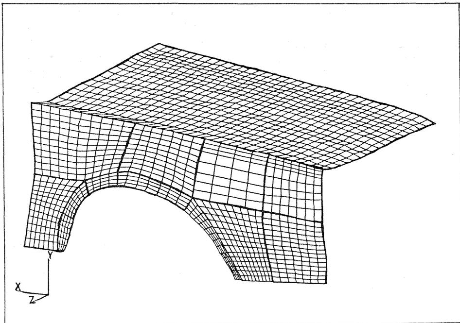
Fig. 2. Patch division and patch networks of car hood part and wheel housing.
