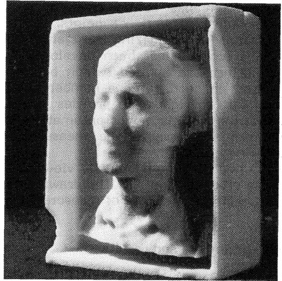
Fig. 4. N.C. milled surfaces of a face.
