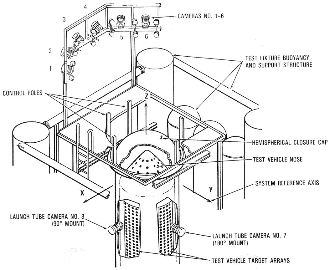
Figure 1: Test fixture assembly
