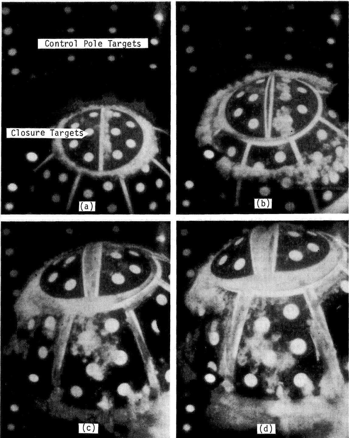
Figure 4: The closure at four epochs during a test event, as viewed from camera #4
