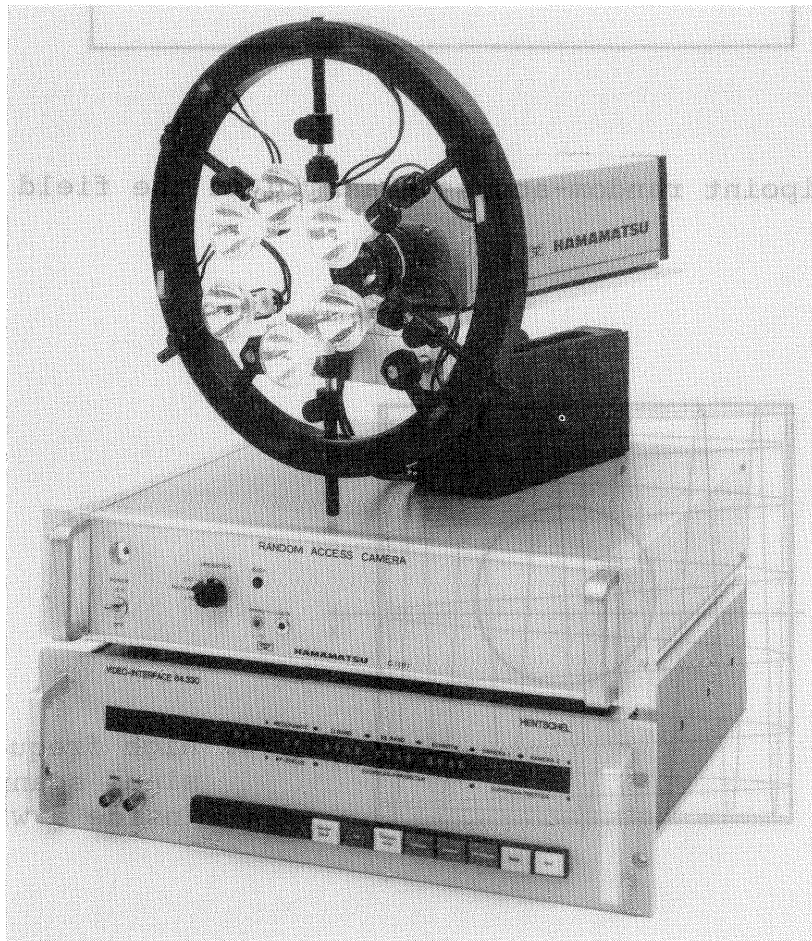
Fig. 2: Hentschel random-access tracking system HSG 84.30 with Hamamatsu camera C 1181. Halogen lamps for illumination of retro reflecting targets
