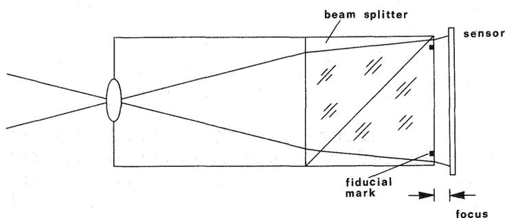
Fig. 5 CCD-camera with fiducial marks, object recording (compare fig. 6)
