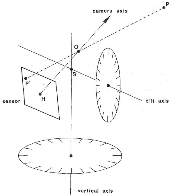
Fig. 1 local sensor orientation by means of the theodolite
