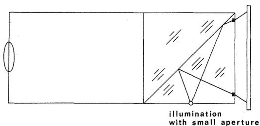
Fig. 6 CCD-camera with fiducial marks, recording of the fiducial marks (compare fig. 5)
