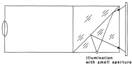
Fig. 6 CCD-camera with fiducial marks, recording of the fiducial marks (compare fig. 5)
