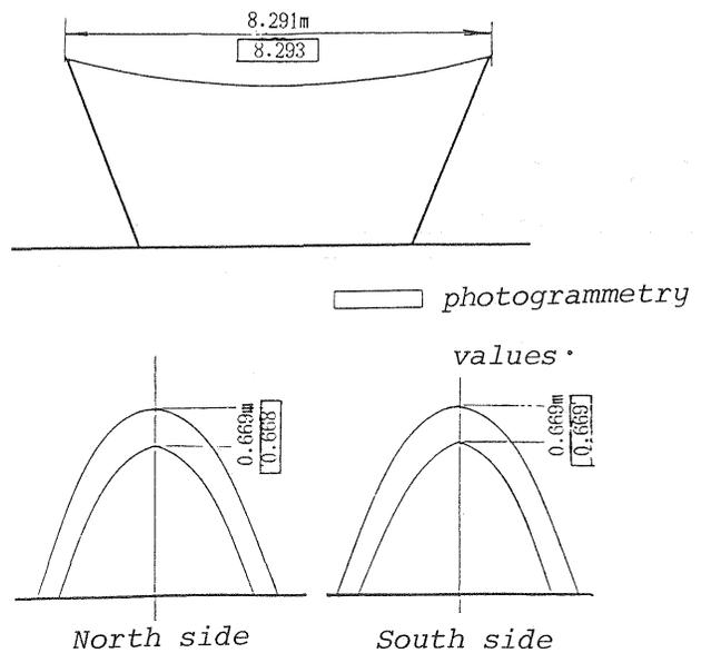
Fig. 6 Comparison of design spec. and photogrammetry data
