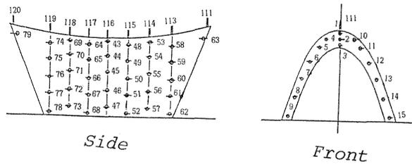
Fig.3-2 Setting position of targets
