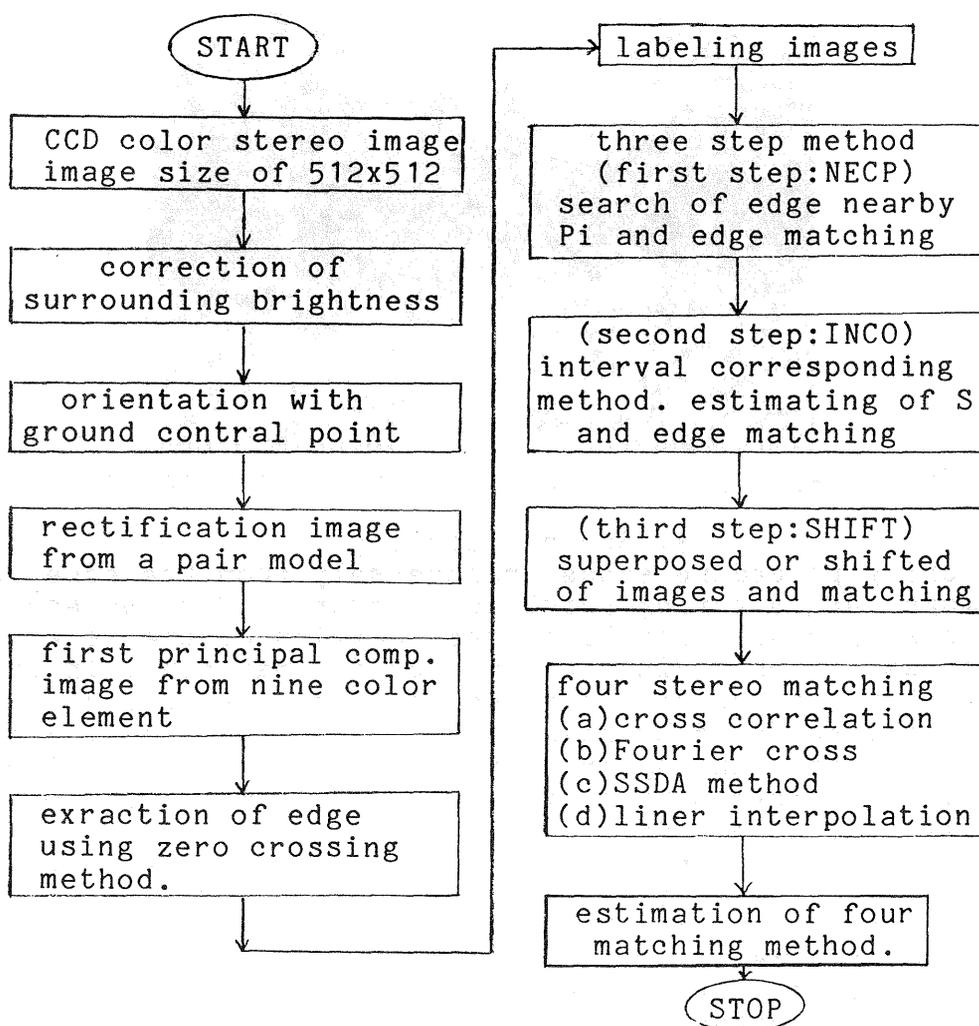
Fig.3-1 processing flow of four matching method
