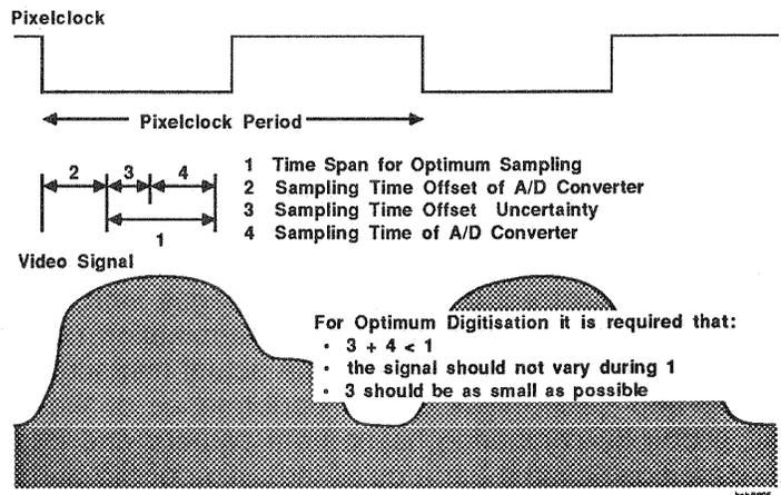
Figure 7: A/D converter timing and video signal
