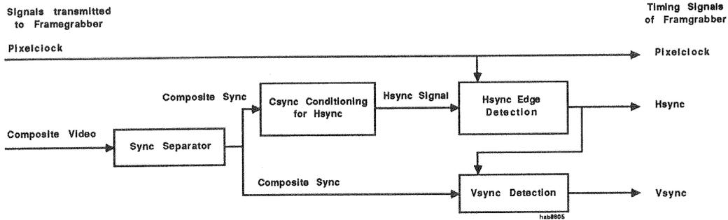
Figure 6: Synchronisation with composite video and pixelclock
