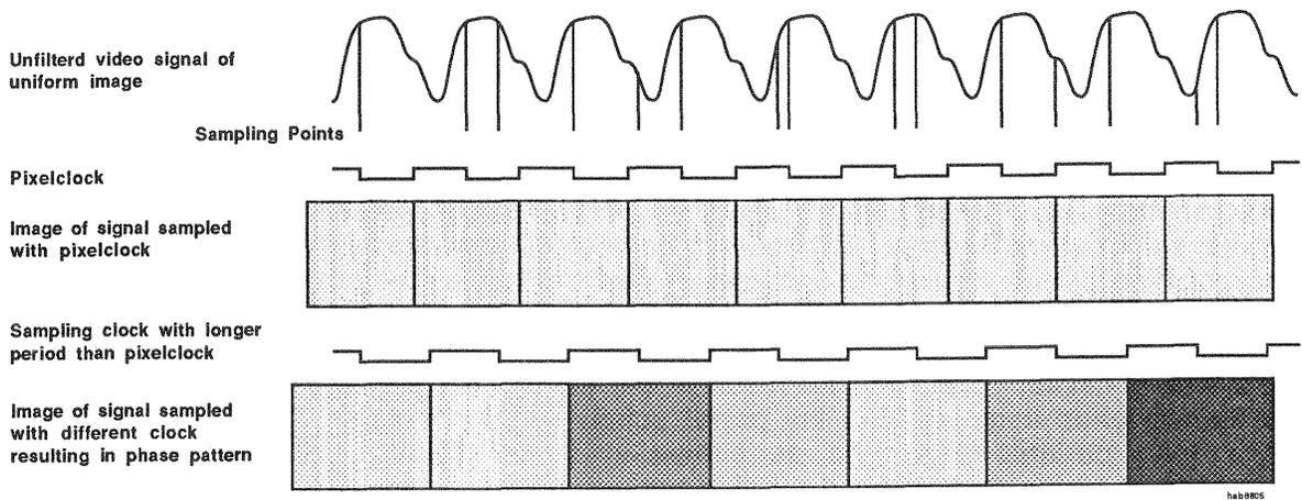
Figure 4: Sampling rate and phase patterns of typical video signal (The drawing is schematic and effects are exaggerated)
