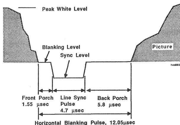
Figure 3: The CCIR video signal: horizontal synchronisation pulse
