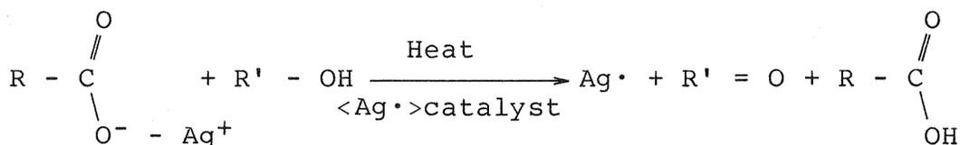
The reduction reaction occurs on all the surfaces of the heated coated layer. However, reaction speeds at exposed areas differ from those at areas not exposed due to differences in the amount of latent image silver. The difference in reaction speed is reflected on the amount of image silver. This forms a photo image.
