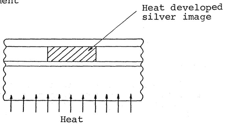
Figure 1 Exposure and development in dry-printing
