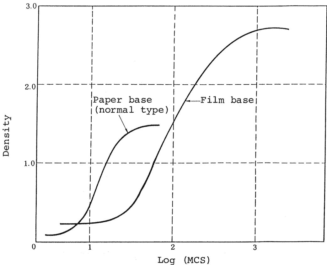
Figure 2 Characteristics curves of photo-sensitive sheets used for dry-printing
