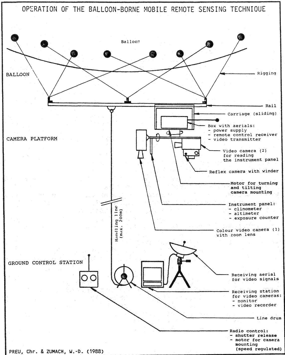
Fig. 1: Operation of the balloon-borne mobile remote sensing technique
