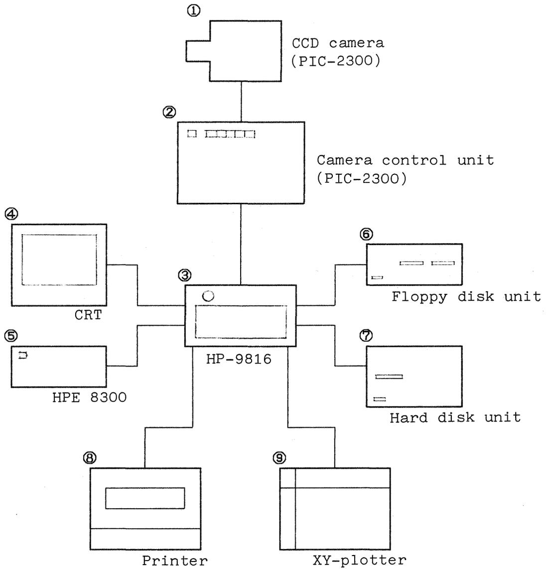
2. Automatic crack analysis system
