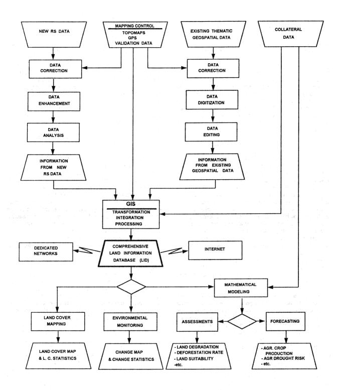
Figure 1: System Flowchart for Coordinated Land Cover Mapping and Environmental Monitoring from RS Data
