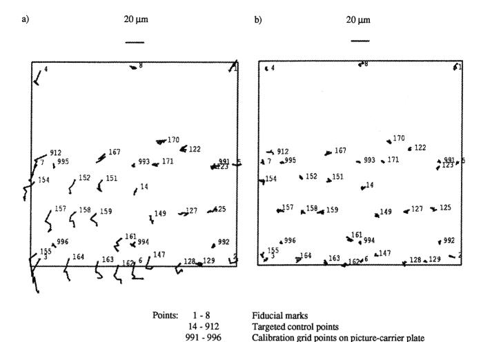
Figure 1. Changes of the picture-carrier coordinates. a) A test where the measurements were started immediately after the system start-up. The light source was the stereoplotter's fluorescent tube. b) A test where special care was taken to reduce the variation of temperature. The light source was placed outside the stereoplotter.
