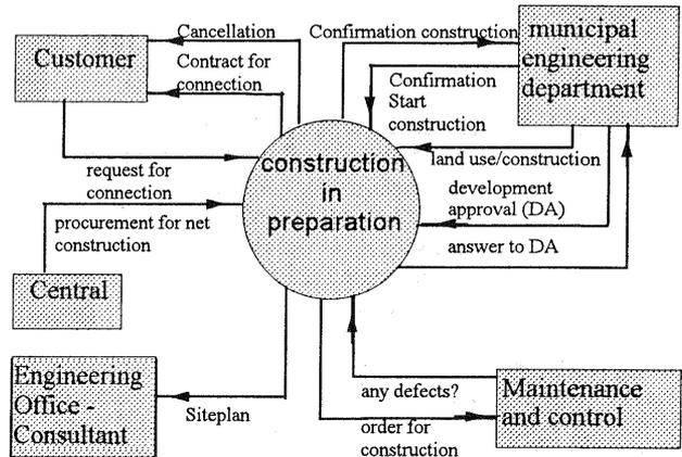
Figure 2: context diagram of a work process of an electric house connection
