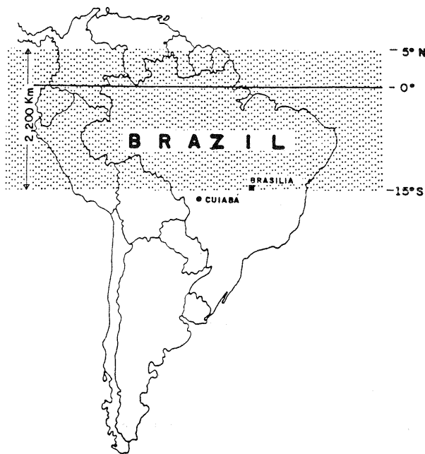
Figure 1. South America and imaged swath by the equatorial orbit of the Brazilian Remote Sensing Satellite (SSR).
