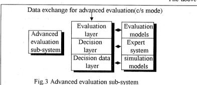
show in Fig. 3, which is used to perform an analysis of basic evaluation data from the first subsystem and to recommend the best basic evaluation decisions or strategies for disaster evaluation application subsystem. The decision and evaluation a models, expert
