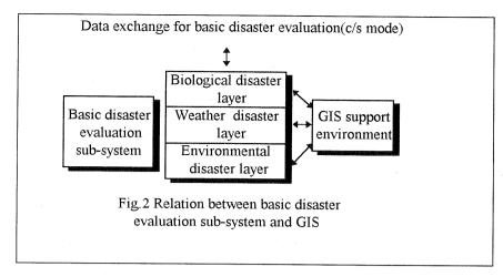
2 and 3. The subsystem is primarily intended to provide the "raw" evaluation service of agricultural disasters which is directly used by an end user and does not support further decisions based on raw evaluation. Two main components such as GIS support environment and Data base management system support its major operations. The second is advanced evaluation subsystem
