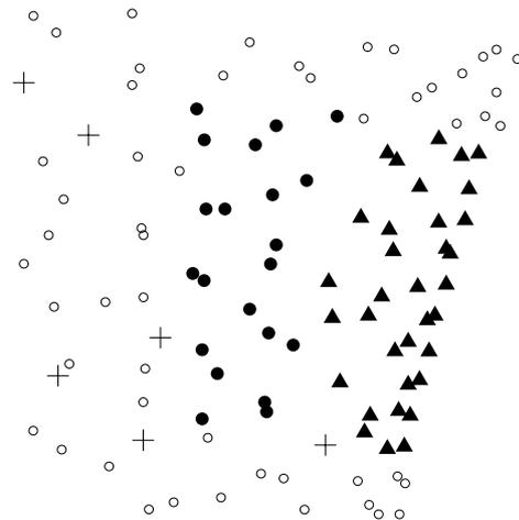
Figure 8: The laser point elevations are grouped into three planar surface patches. Solid circles and solid squares identify points that are likely to belong to a roof plane. The crosses are points on the ground that may lie on a horizontal surface. Grouping did not classify the points depicted as triangles.
