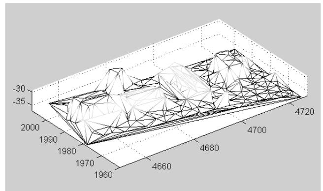
**Figure 5. New surface using breaklines and laser data.**
