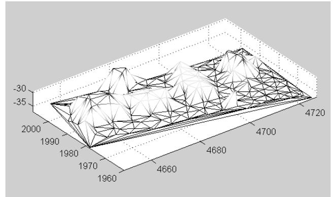
**Figure 4. Surface from laser data.**
