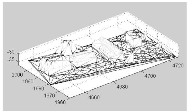
**Figure 6. Incorporation of vertical projection of roofline to ground surface.**
