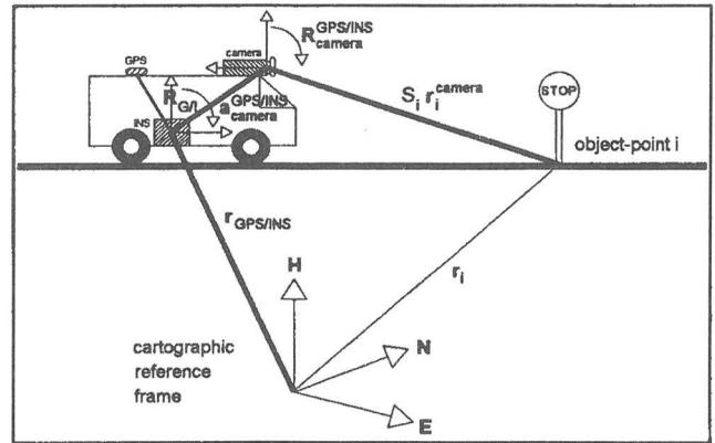
Figure 1: Unified model for a georeferencing procedure
