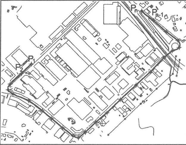
Figure 5: Determination of the trajectory of a MMS by a cubic spline applied to points acquired from a digital map
