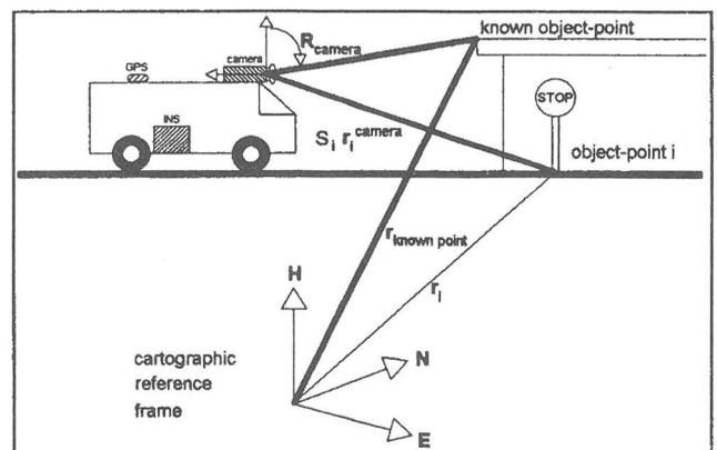
Figure 2: Alternative model for the georeferencing procedure
