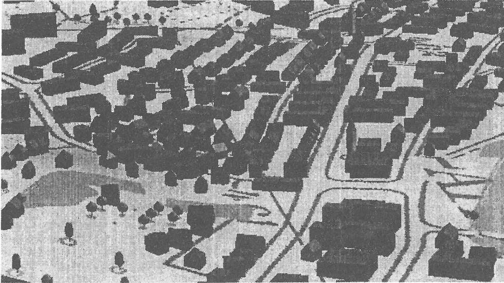
Fig. 5 Combination of planimetry, DTM and three-dimensional objects
