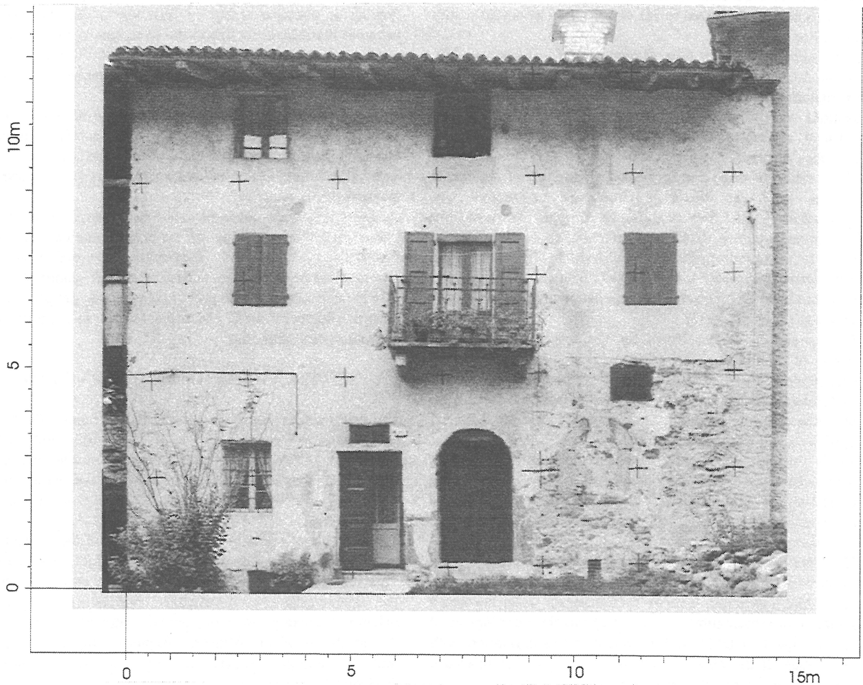
Fig. 2 - Raster imaging of the main façades for a building (ortogonalisation, scaling, mosaicking and georeferencing).
