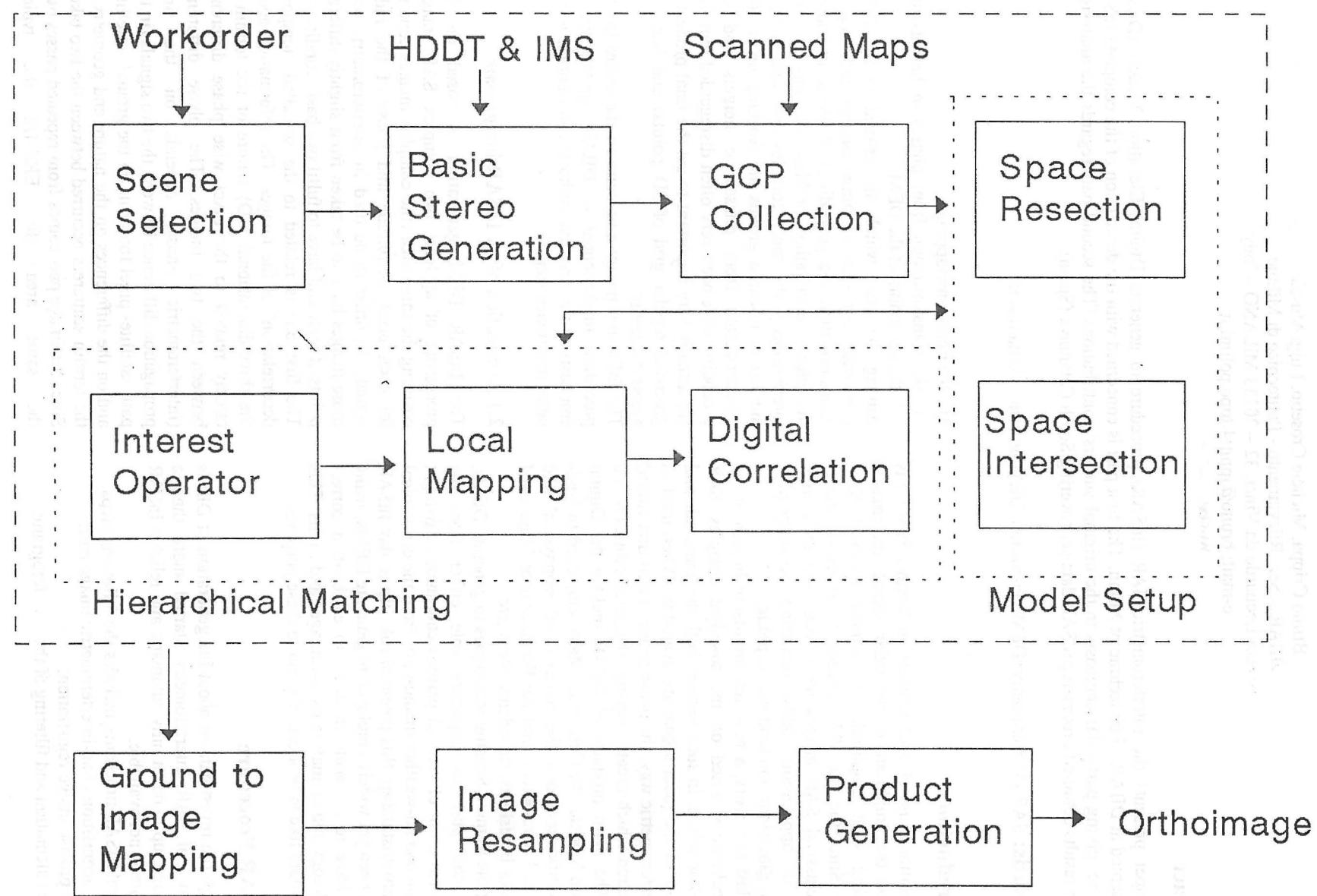
Figure-1 : Schematic Diagram of Orthoimage Generation
