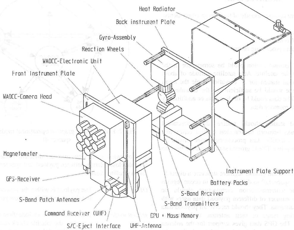
Fig.4: Integration scheme I of the micro satellite
