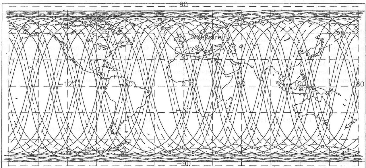
Fig. 1: Coverage of one day by the ocean color imager (FOV = 60°) within the 600km x 600km circular Sun-synchronous orbit
