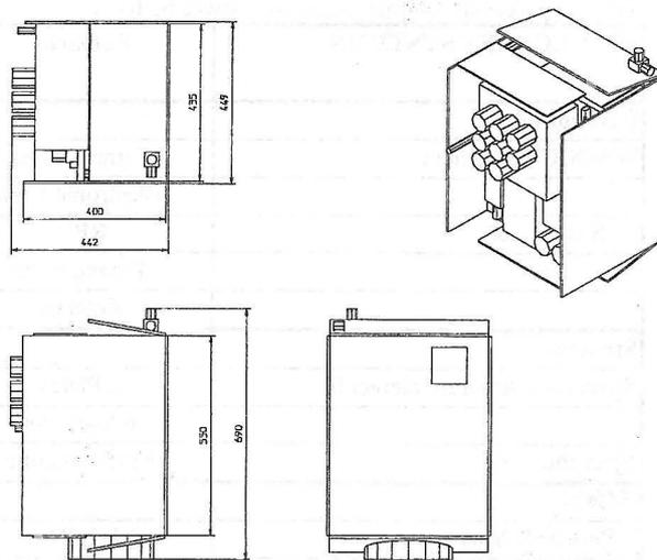
Fig.2: Launch configuration of the micro satellite
