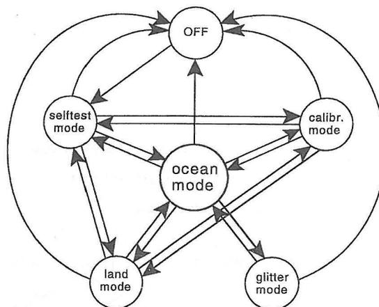
Fig. 7: Reduced state graph of operational modes of the spacecraft
