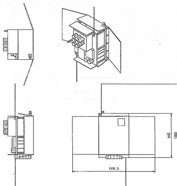
Fig.3: Flight configuration of the micro satellite
