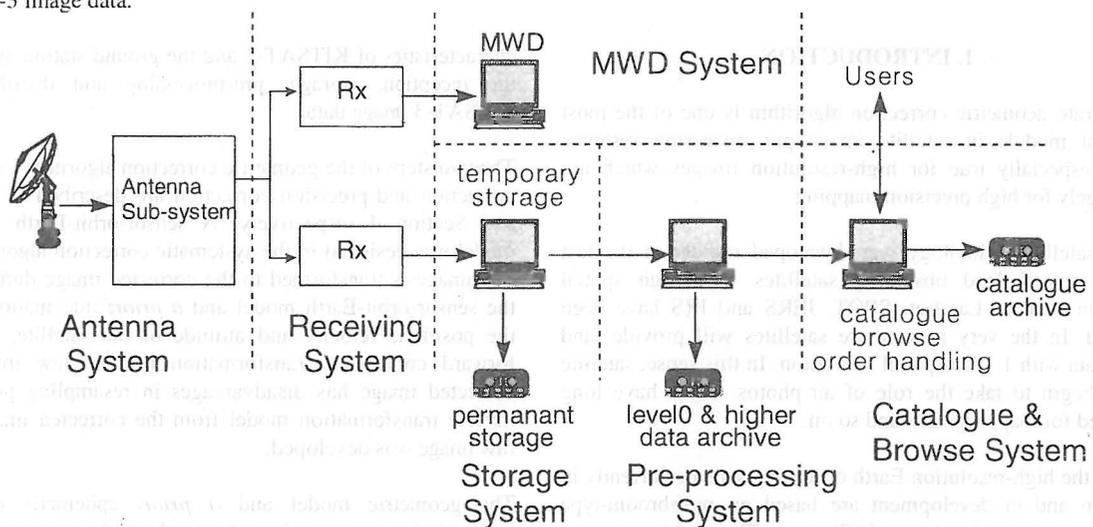
Figure 1. KITSAT-3 image data handling systems
