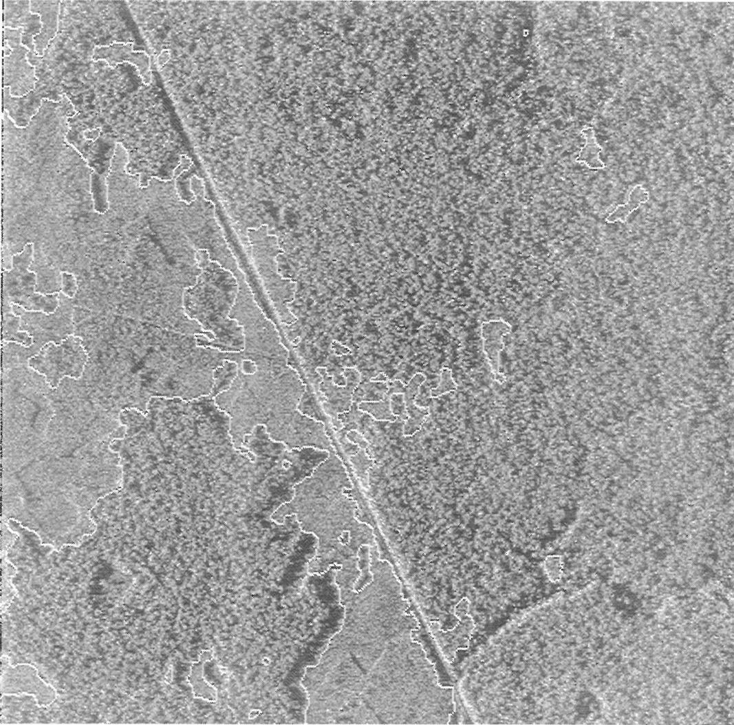
Figure 5: Identification of clearing in the Brazilian rainforest. The original image was processed by a 7 by 7 mask to provide an image of normalised log estimates. This image was processed by the annealing segmenter and then thresholded. Finally, the resulting edge map was overlaid on the original data.
