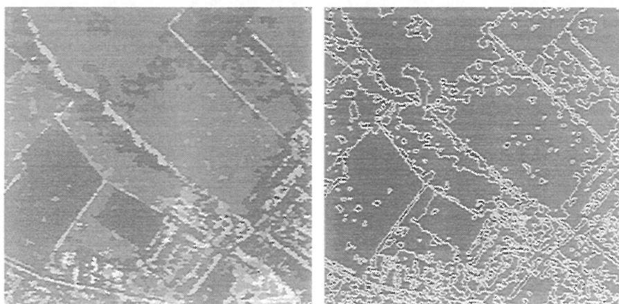
Figure 3: Annealing classification and edge map for the SAR image of figure 2
