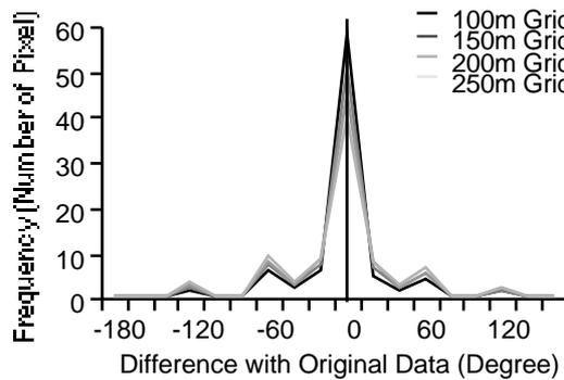
Figure 2. Accuracy of Slope Aspect according to Spatial Resolution
