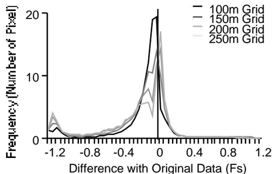
Figure 7. Accuracy of Safety Factor according to Spatial Resolution
