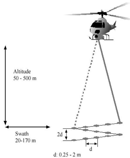
Figure 1 Normal flying and data acquisition conditions for Saab TopEye
