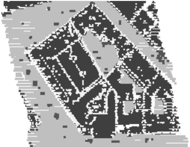
Figure 13 LRF data automatically labelled by MDL using the cost function described in 3.2 as ground, vegetation and buildings with breakpoints.
