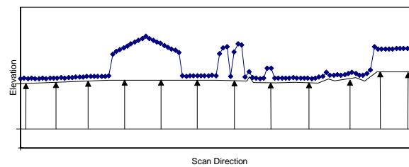
Figure 3 Connecting ground surface to LRF data
