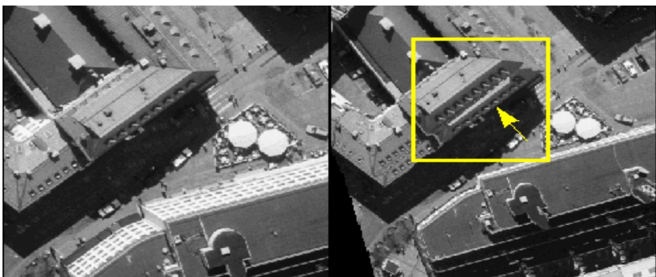
Figure 8: Original perspective image to the left and generated orthophoto to the right. The vertical walls of the buildings have disappeared on the rectified image. The area of the street that is occluded in the middle of the image results in a projection of the roof on the street that looks like a double row of roof windows.
