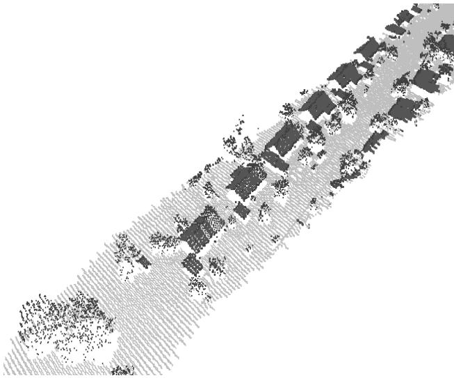
*Figure 14 Classification of site 2. The separation of the three classes is fairly successful. Single scan lines erroneously classified can be seen at some buildings. Some of them are due to chimneys and other objects disturbing the statistic variables.*
