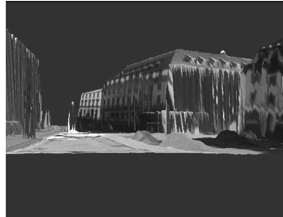
Figure 10: Perspective view of DEM together with image information. Note that the form of the roof windows is preserved fairly accurate. The windows on the houses on the right side is visible while the left ones are occluded in the image, see figure 5. The bumps in the foreground are cars.
