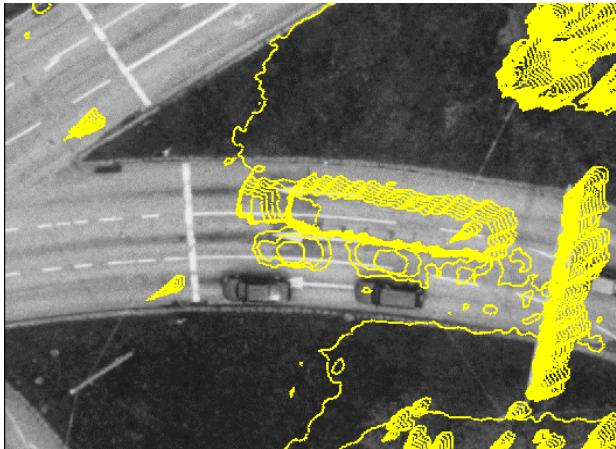
Figure 15 Range data of truck visualised with contour lines.
