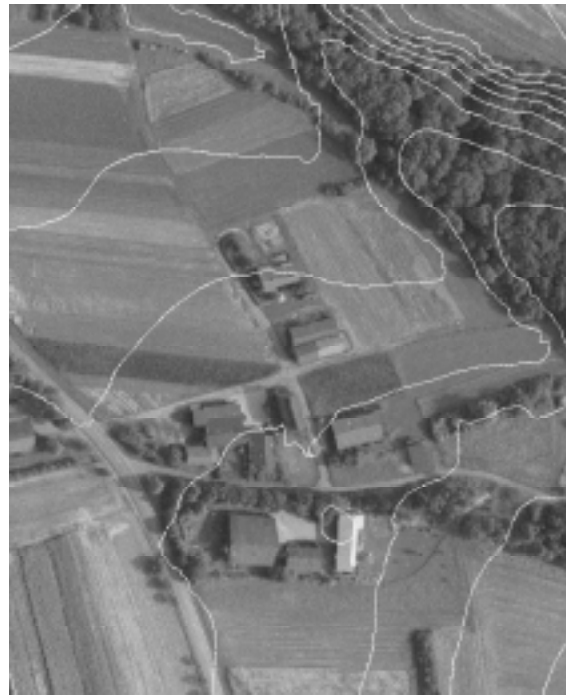
Figure 10: Contour lines derived from DTM after filtering and smoothing
