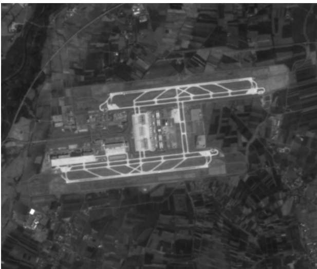
Figure 5: Zoom into the orthophoto of forward looking channel (pixel size 20m, airport Munich)
