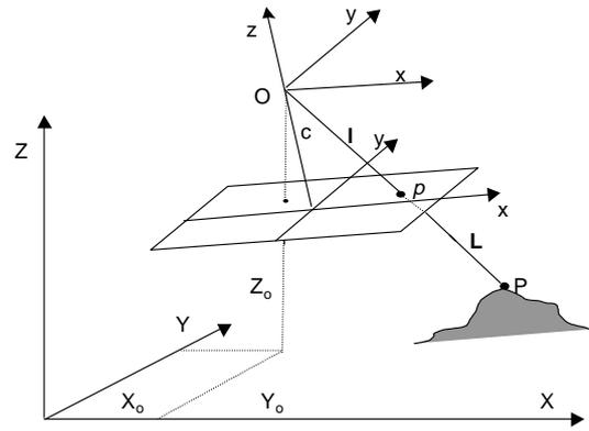
Figure 1. Reconstruction of the projective ray passing through the point image, projection center and terrain point.
