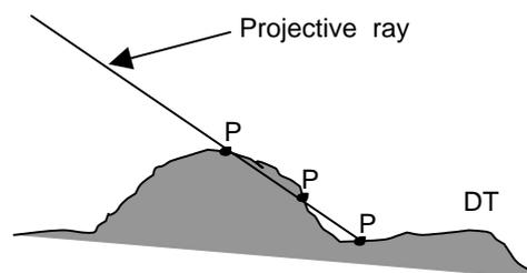
Figure 2: Critical Intersection of projective ray and DTM
