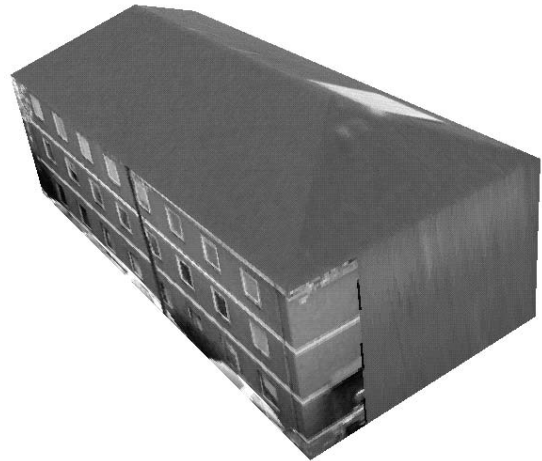
Figure 16: Texture extraction example. The texture is automatically extracted and mixed from two aerial images (figure 14) and one close range image (figure 15). Please note, that the wall to the right is only partly covered by the close range image and thus only partly mapped with texture from that image.
