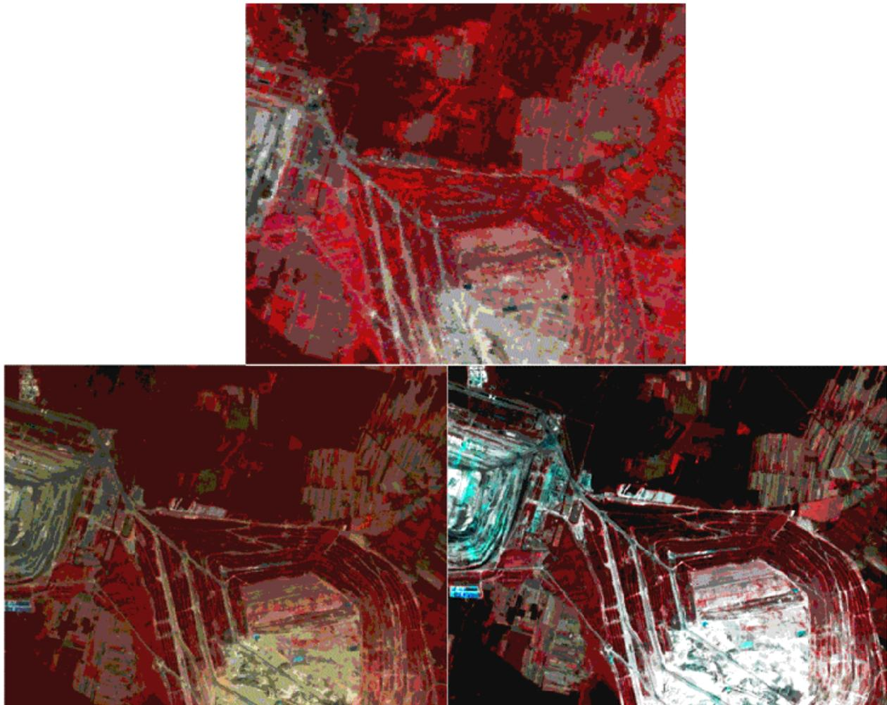
Fig. 7. Merging of LANDSAT TM (4 3 2) and SPOT PAN images (IHS transformation)
