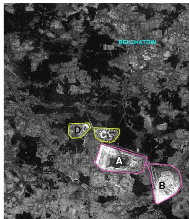
Fig. 1. SPOT PAN image over the study area (A - open-pit-mine; B - dump area; C - electric power plant complex; D - slag&ashes containers)
