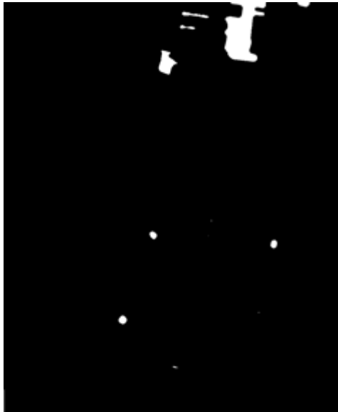
Figure 4. Changes detected from Figure 3b. The Figure 3b image was transformed into a binary image and then the noise was removed from a simple noise reduction filtering.
