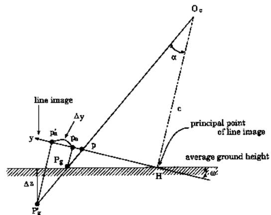
Figure 3: Image error from height differences.
