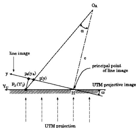
Figure 5: Geometry of Level-2 imagery.
