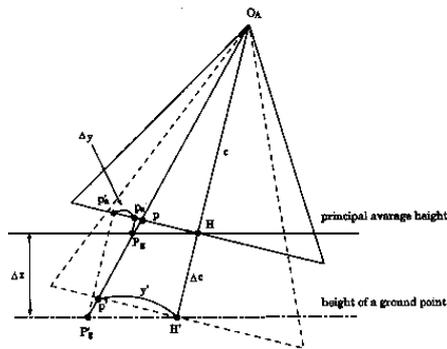
Figure 4: Correction of image conversion error.
