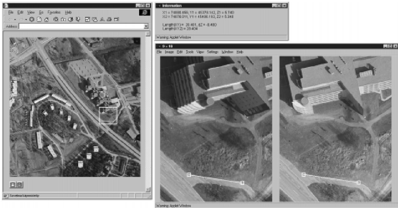
Figure 3. A typical layout of the windows used in WebTop photogrammetry. The window on the left is a browser window displaying an overview image. The window on the left has been opened by a Java applet and contains a stereo imagery for the area in interest. A measured distance is displayed there also, the other measurement data being displayed in a separate window on the top.
