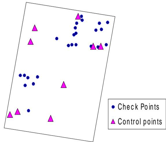
Figure 2: Distribution of control and check points within the test area.
