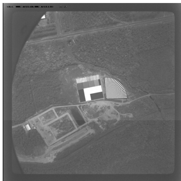
Figure 13. 4K by 4K AIMS™ image of space resolution target range at NASA Stennis Space Center.
