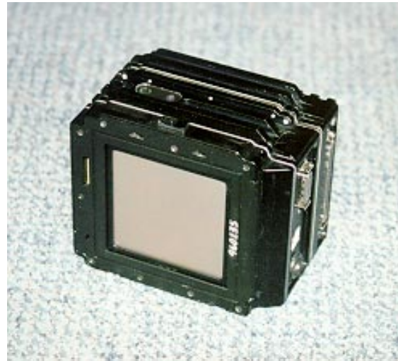
Figure 3. 4K by 4K BigShot™ camera-back.
