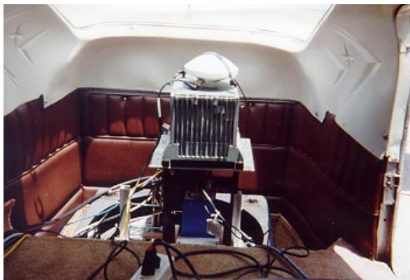
Figure 2. LN100 INS installed in an aircraft.
